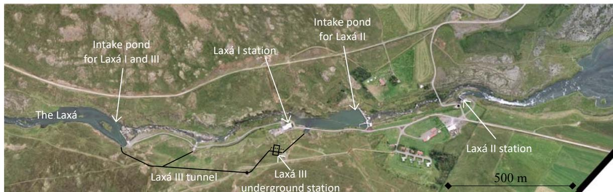
*Fig. 1. Map showing the Laxá Hydropower Plants within the Laxá Canyon.*
