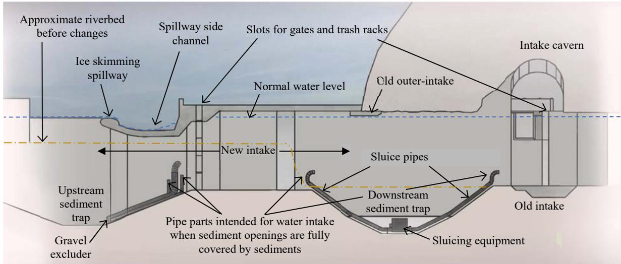
Fig. 5. Longitudinal cross section through the old and new intake.
